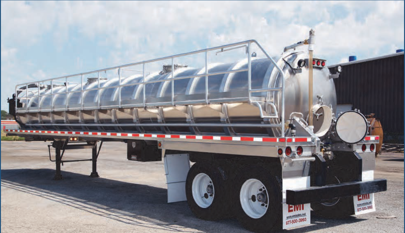
150 Barrel Aluminum Vacuum Trailer with Air-Ride Suspension, full catwalks with rear entrance.
